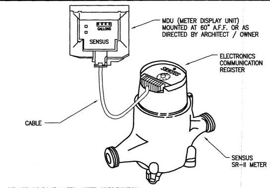
REMOTE READOUT WATER METER SPECIFICATION
