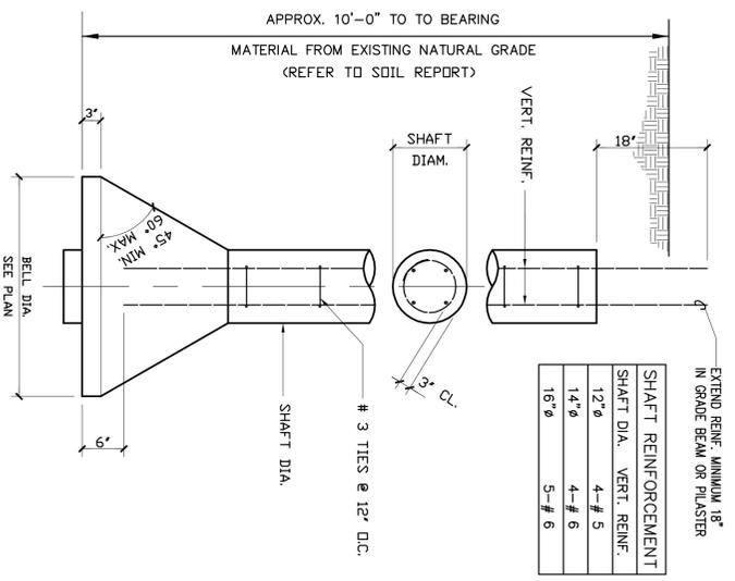
**TYPICAL DRILLED PIER DETAIL**
